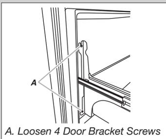
A. Loosen 4 Door Bracket Screws
