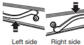
2. Place a broad, flat container beneath the drain pump filter to collect the drain water. Release the black hose from the hose clip, remove the plug, and drain the hose into the container. Empty the container. Repeat this procedure if necessary until all the water has drained. Make sure that the black hose is completely dry, replace the plug, and secure the hose in the clip.
