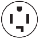
4-wire receptacle (14-30R)
