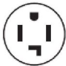
4-wire receptacle (14-30R)
